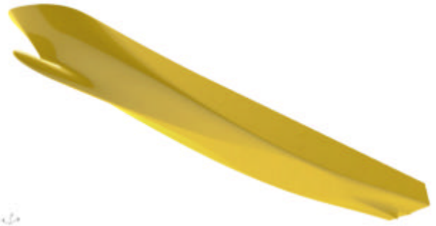
Figure 9: LSHF - Hull form optimised for the lower speed
