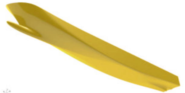
Figure 10: HSHF - Hull form optimised for the higher speed
